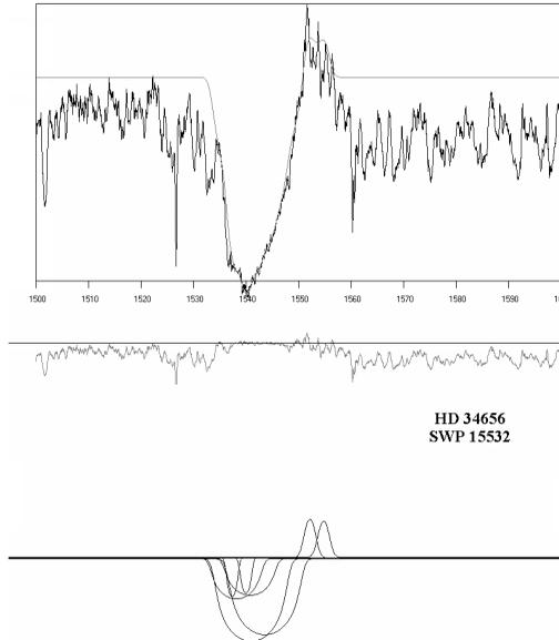
**FIGURE 1.** The C IV resonance lines ( $\lambda\lambda$  1548.155, 1550.774 Å) in the spectrum SWP 15532 of HD 34656. Each of C IV spectral lines consists of three SACs and one emission component. The graph below the profile indicates the difference between the fit and the observed spectral line. Below the fit one can see the decomposition of the observed profile to its SACs.
