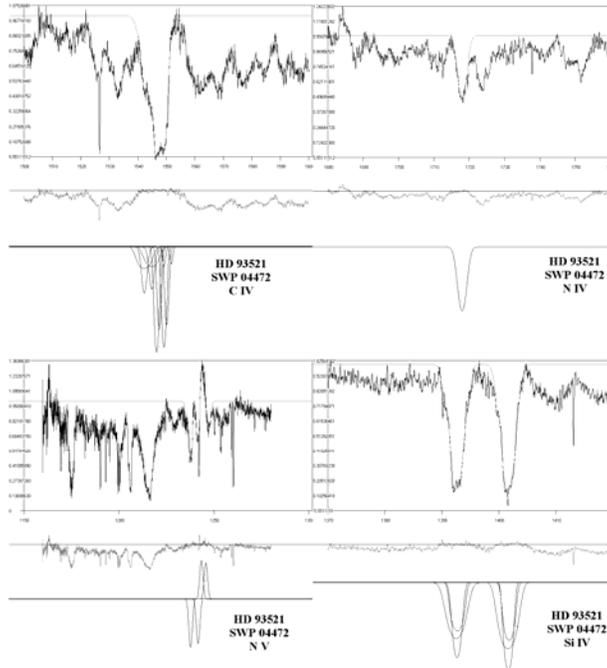
**FIGURE 8.** Best fit of the C IV, N IV, N V and Si IV spectral lines of the Oe star HD 93521. The graph below the fit indicates the differences between the observed spectrum and the fit. Below the fit one can see the analysis of the observed profile to its SACs.
